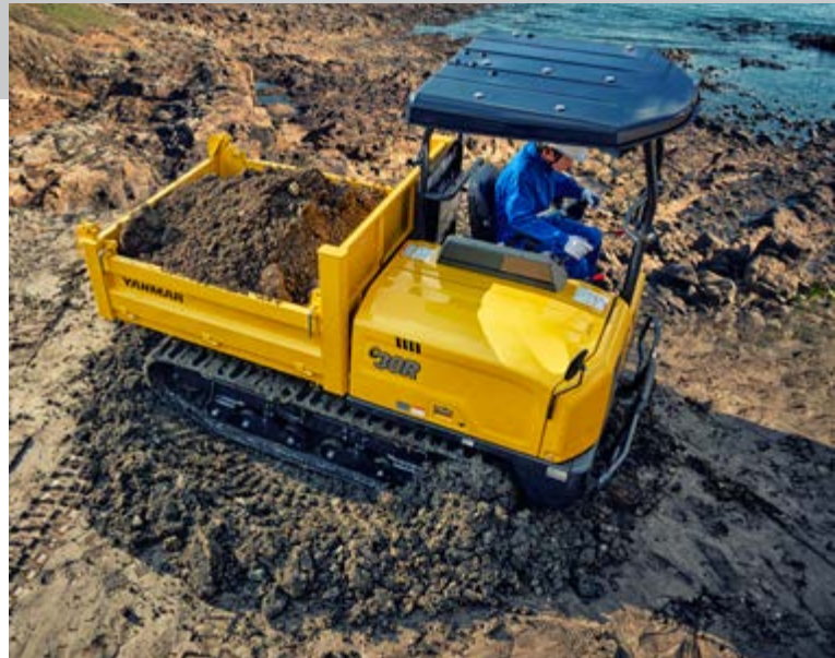
Spin turn by reverse turning both crawlers
