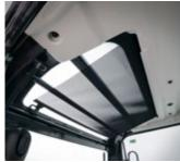
The roof window of the SV60 is protected by a fully integrated sunshade for a maximum comfort.
