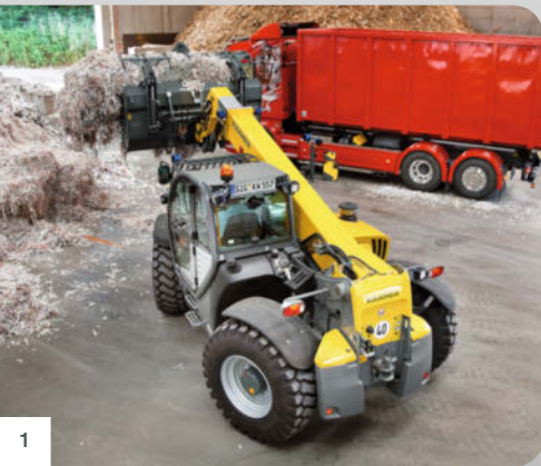
1 Easily reach every corner: Kramer telehandlers with all-wheel steering effortlessly drive into the smallest spaces.
