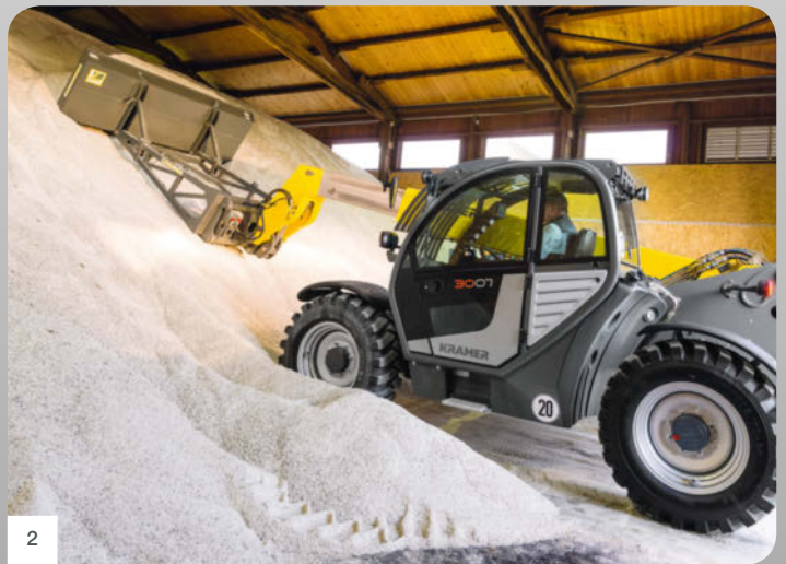
2 Protection against loss of value: The additional corrosion protection was specifically designed for use with aggressive media, such as salt and fertilisers.
