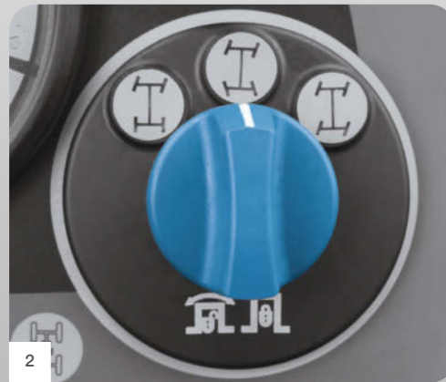
2 Simple and intuitive: Quick change of the steering mode via rotary-push button.
