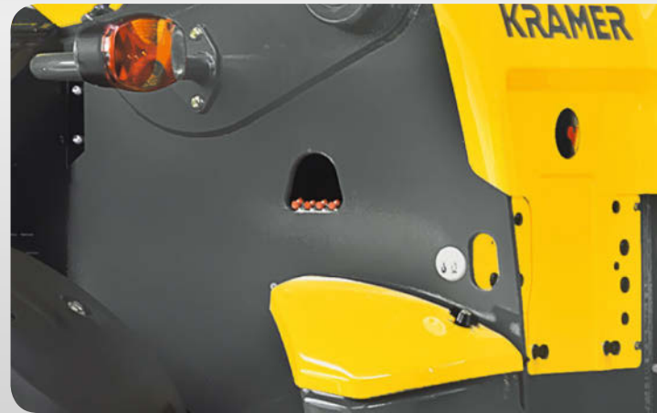
Joint lubrication points: Oscillating axle, lifting and balance cylinder can be lubricated in one operation. It is not necessary to lift the telescopic arm.
