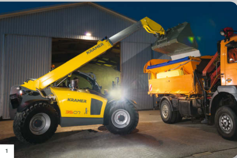
1 Brighten dark winter days: On request, the machine is equipped with up to eight LED headlights with an output of 2,200 lumens each.
