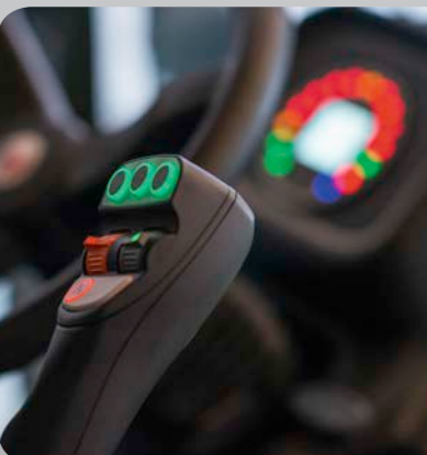
Sensitive and precise control of the machine and attachment via hydraulically activated, pilot-operated joystick.
