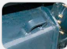
Fixing points on track frame and blade to facilitate transportation on trailers
